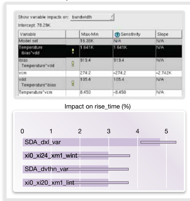
Figure 10: Variation Designer provides PVT sensitivities and Monte Carlo impacts, revealing causes of variation problems with no additional simulations.
