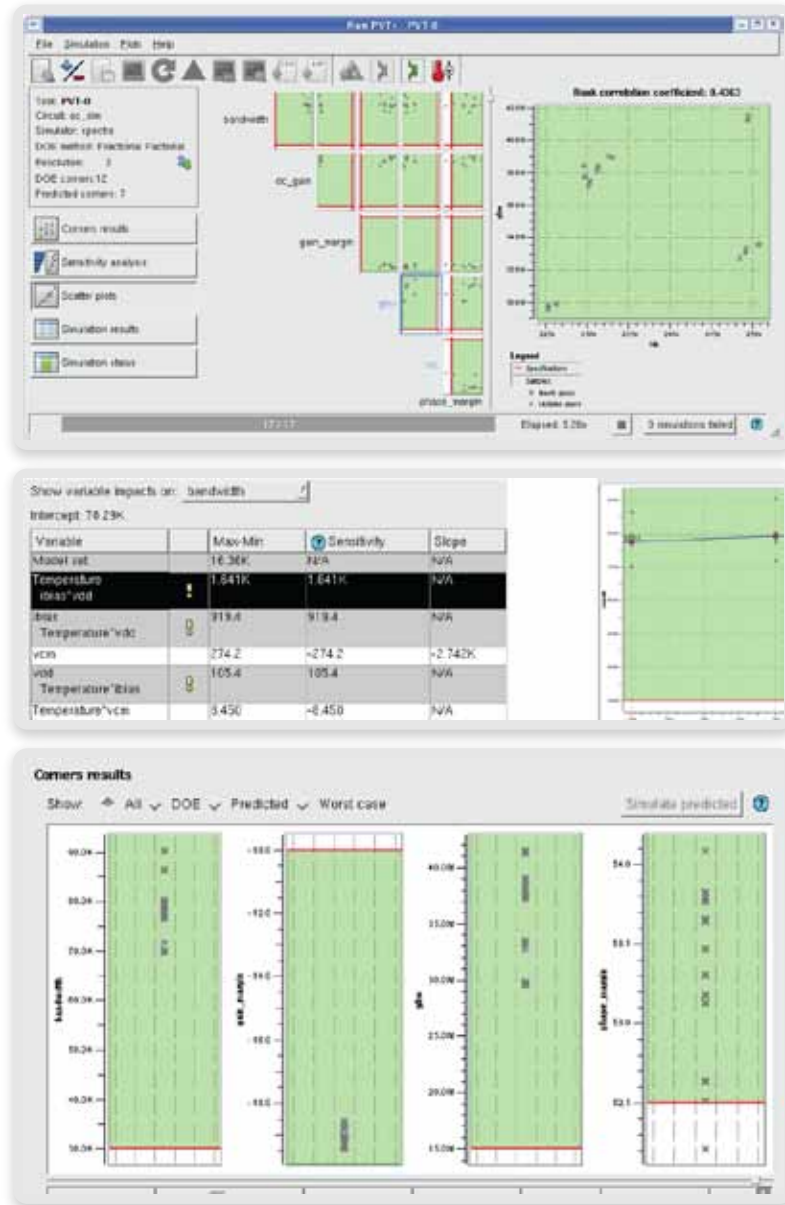
Figure 5: Variation Designer's PVT visualizations help to see the effects of variation clearly without the need to post-process data manually or to generate plots with third party tools.
